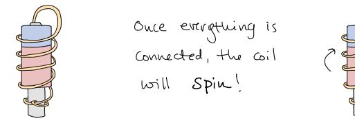
WHY Does THIS HAPPEN? Current flows through the battery, through the wire, to the magnet attached to the other end of the battery, creating a closed circuit. The Loventz force, a force which acts on moting charges in the presence of a magnetic field, is what causes the Gil to turn! Force (out of the page) (into the page) Current Flowing N LOVENTE FORCE!
